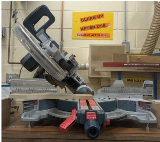
Work Piece Secured Horizontally Against The Table (2" Max Height At 45°, 10" Max Depth)
