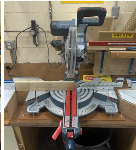
Work Piece Secured Vertically Against The Fence (7" Max Height, 7-1/2" Max Depth At 45°)
