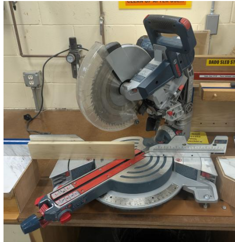
Work Piece Secured Vertically Against The Fence (7" Max Height, 7-1/2" Max Depth At 45°)
