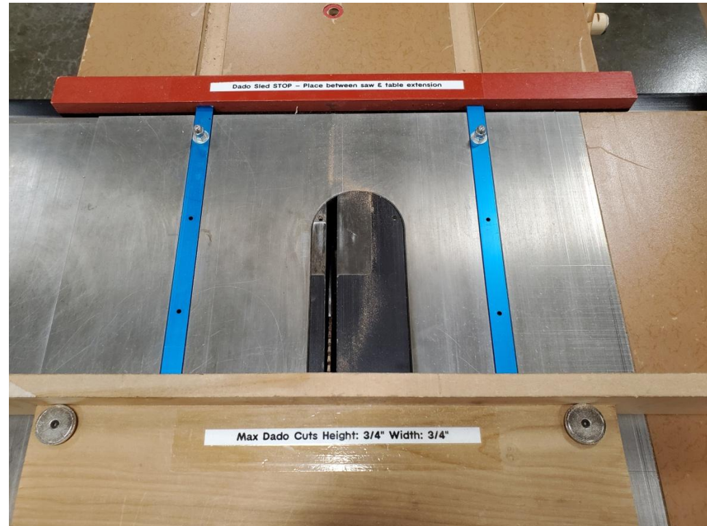
Dado blades not installed for this photo
