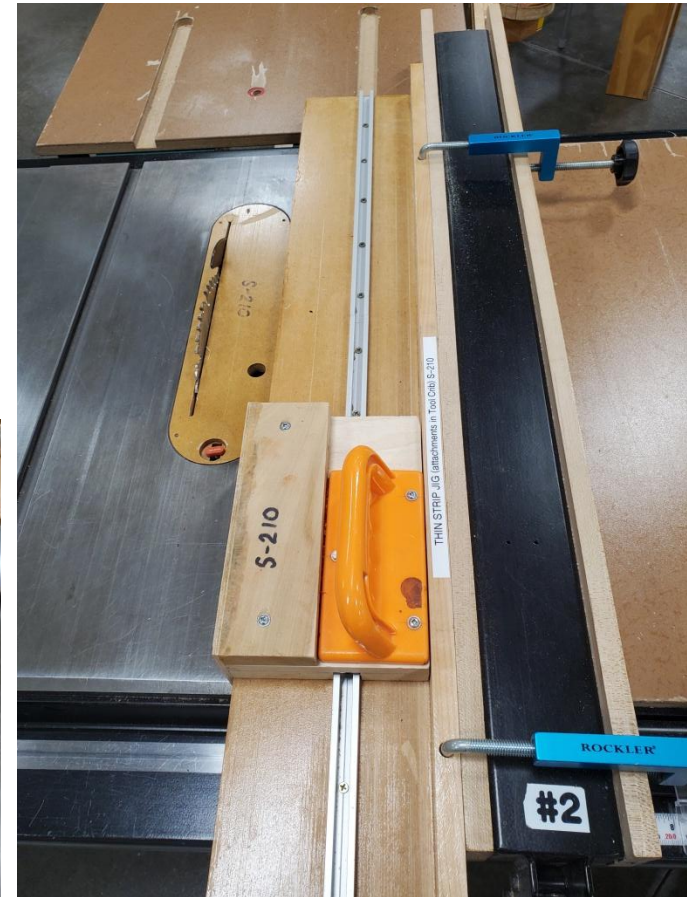
Shown with riving knife instead of blade guard assembly for clarity
