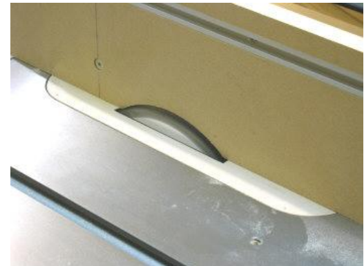
Sacrificial Fence attached to primary fence for rabbets
